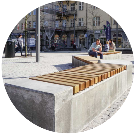
11 Concrete & Timber Bench: Concrete seatwall / retaining wall with timber bench
